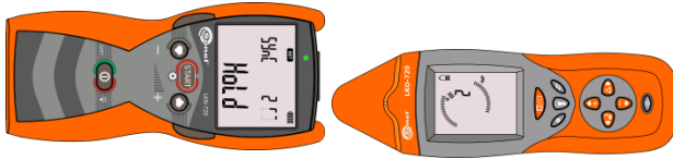
Fig. 5 Positioning the transmitter and receiver during synchronization
