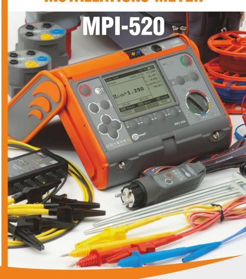
The MPI-520 multifunction meter is dedicated to perform diagnosis of electrical installation according to IEC 61557 standards. Digital meter MPI-520 is designed to measure impedance of a short cicuit loop also without triggering RCD, parameters of RCD, insulation resistance, earthing resistance, continuity and also for phase sequence testing. Furthermore it is used for measurement of AC voltage and current, frequency and power.
