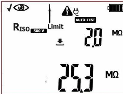
Positive visual inspection result. If the **AUTO-TEST** (**AUTO-TEST**) mode is on, the tester will automatically run the subsequent tests, which by default is: **Riso**. If the **AUTO-TEST** mode is off the tester will wait for the **START/STOP** button to be pressed. At this stage it is possible to return to the previous test
