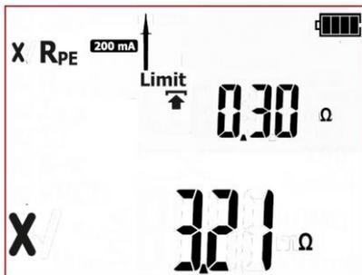
Inorrect result. The value of PE resistance is above the set limit. Red LEDs of FAIL indication are on.
