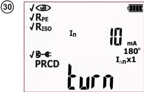
Switch on PRCD. Tester will commence the first measurement. If PRCD trips, a message prompting to switch on the RCD will be displayed on the main screen: 'turn on PRCD'.
