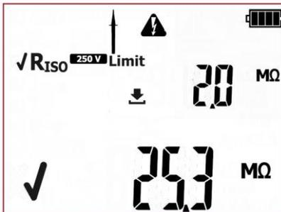
Correct result. The value of insulation resistance is above the set limit. Green LEDs of PASS indication are on.
