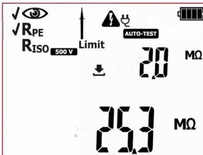
Measurement of PE protective conductor has been completed. If the measurement result is negative, further measurements will not be conducted. In case of the positive test result: If the **AUTO-TEST** mode is on, the tester will automatically run the subsequent test, which by default is: **R<sub>iso</sub>**. If the **AUTO-TEST** mode is off the tester will wait for the
