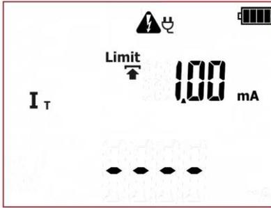
The tester is in touch leakage current measurement mode.
