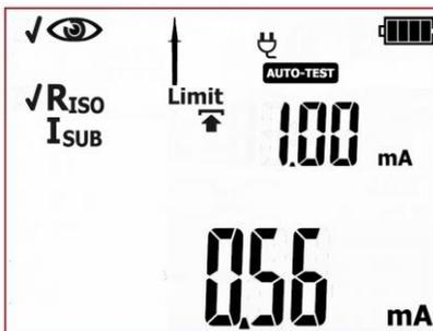
Measurement of **Riso** insulation resistance has been completed. If the measurement result is negative, further measurements will not be conducted. In case of the positive test result:
