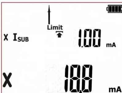
Incorrect result. The value of leakage current is above the set limit. Red LEDs of FAIL indication are on.
