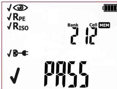
A cell occupied by AUTO test, IEC or PRCD test result (corresponding icons for subsequent tests, along with results are displayed on screen).
