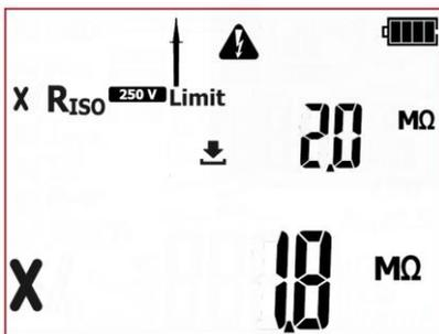
Inorrect result. The value of insulation resistance is below the set limit. Red LEDs of FAIL indication are on.
