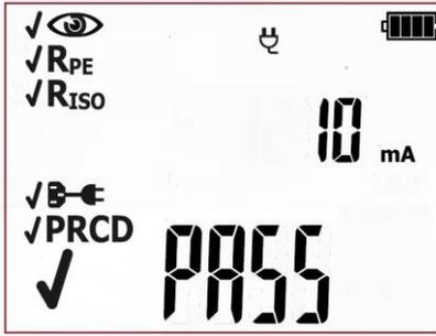
Correct result. The result of each single test of the sequence is positive. Green LEDs of PASS indication are on.
