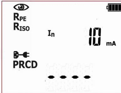
The tester is in PRCD trip time measurement mode.
