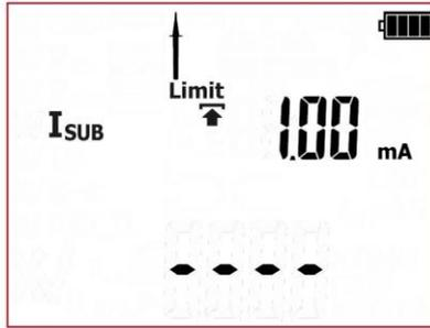
The tester is in substitute leakage current measurement mode.
