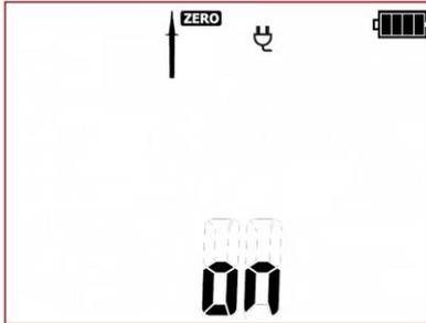
The compensation value has been measured. 0Ω is displayed on the screen, along with the permanent **ZERO** symbol. After 3 seconds the tester returns to measurement mode. The active test lead compensation is indicated by **ZERO** icon being displayed on screen during the tests of R<sub>PE</sub> (200mA, 10A) and CL I autotests. The compensation resistance will be taken into account then displaying test results of R<sub>PE</sub>.
