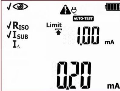
Measurement of substitute leakage current has been completed. If the measurement result is negative, further measurements will not be conducted. In case of the positive test result: If the **AUTO-TEST**
