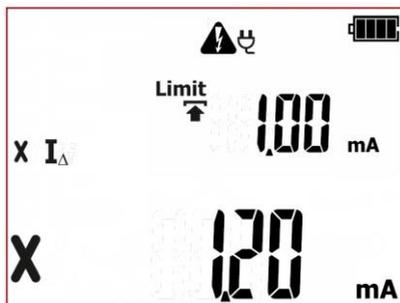
Inorrect result. The value of leakage current is above the set limit. Red LEDs of FAIL indication are on.
