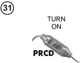
PRCD must be switched on every time after it trips. Each consecutive measurement will be performed automatically. The tester will wait for 2 minutes for the PRCD to be turned back on. After this time, when any of the following occurs: PRCD is not switched on, the circuit is damaged, the FAIL button is pressed, the tester indicates lack of continuity on the measured circuit - the test result will be negative.
