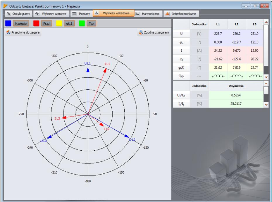
**Fig. 45. Phasor diagram for wye connection.**
